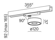
Tolerance for dimensions ± 1mm
