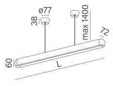
Tolerance for dimensions ± 1mm
