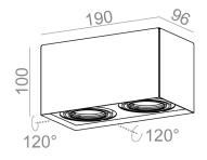
Tolerance for dimensions  $\pm 1 \text{mm}$
