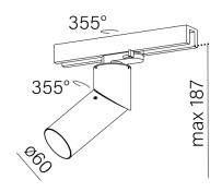
Tolerance for dimensions ± 1mm
