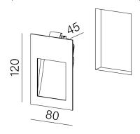
Tolerance for dimensions ± 1mm
