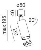
Tolerance for dimensions ± 1mm
