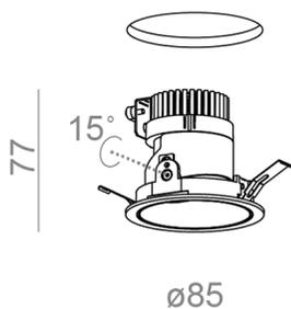
Tolerance for dimensions  $\pm 1$ mm
