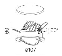
Tolerance for dimensions ± 1mm
