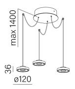
Tolerance for dimensions ± 1mm
