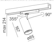
Tolerance for dimensions  $\pm 1$ mm
