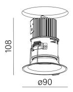
Tolerance for dimensions ± 1mm
