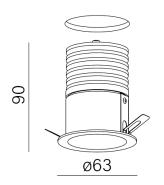
Tolerance for dimensions ± 1mm
